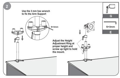
Put on Arm Support to the pole above the Height Adjustment Ring.
