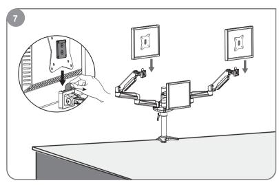
Lift the VESA plate along with monitor and put it on head slot.
