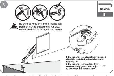
Use a hex wrench to adjust the height tension of the gas spring arm, to keep different weight of monitors still at any position.
