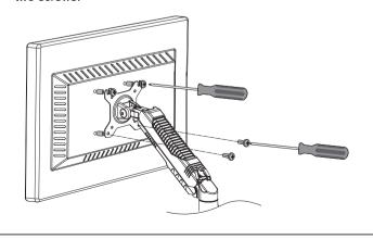
Flush surface installation: Install the upper two screws and
