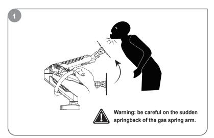
Tear off the cable tie and rebound carefully.
