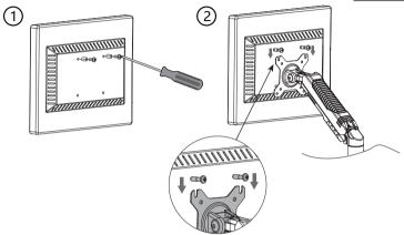
Recessed surface installation:Put spacers between headplate and monitor. Install the lower two screws and fasten the upper two screws.
