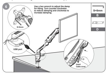
Insert cables into cable covers. Leave enough slack of cables at arm joints for full adjustment.
