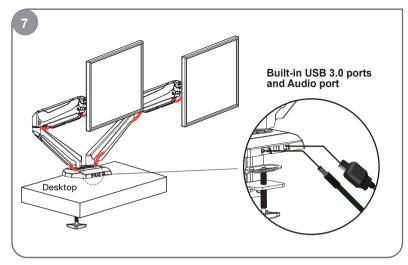
Leave enough slack in the cables at arm joints for full adjustment.
