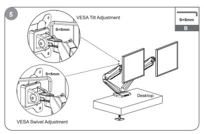
Tighten the bolt with the Allen Key to make the tilt and swivel adjustment.
