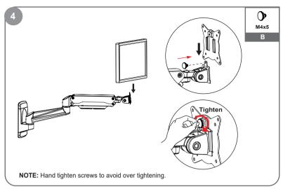
Insert the monitor along with the VESA plate to the arm and lock it. Make sure the security bolt (B) is installed before you rotate the monitor.
