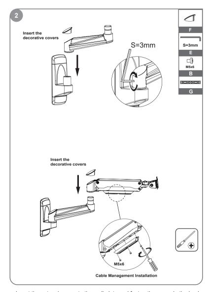
Insert the extension arm to the wall plate and fasten the screw in the back. Insert the gas spring arm above the extension arm.
