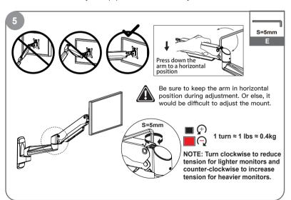
Use a 5mm hex wrench to adjust the height tension of the gas spring arm, to keep different weight of monitors still at any position.
