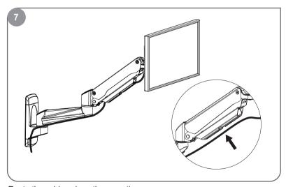
Route the cables along the mounting arms. Leave enough slack of cables at arm joints for full adjustment.
