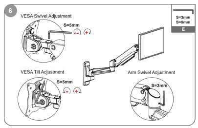
Tighten the bolt with the Allen Key to make the tilt and swivel adjustment.
