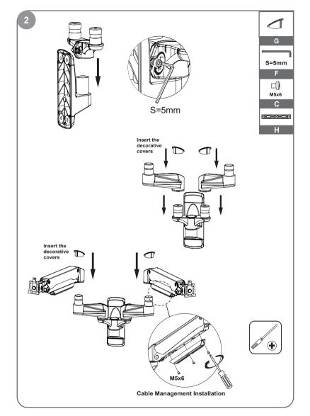
Insert the extension arm to the wall plate and fasten the screw in the back. Insert the gas spring arm above the extension arm.
