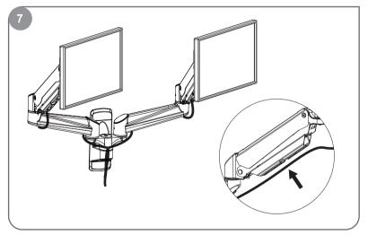
Route the cables along the mounting arms. Leave enough slack of cables at arm joints for full adjustment.
