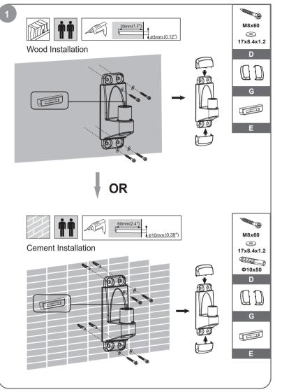
Use a pencil to mark where you will install the mounting base on the wall. Make sure the wall structure can support the weight of the monitors as well as the mount. Also make sure to avoid electrical wiring when choosing where to create mounting holes.
